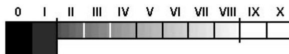
A schematic picture of a zone scale from 0 to X. The border between black and almost black is marked between zone I and II (zone I 1/2). The border between white and almost white is between zone VIII and IX (zone VIII 1/2).
