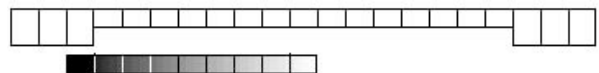
The ideal exposure is to place all the tones of the object except all black, just within the film's threshold to the left.
